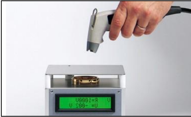
Figure 9. Charge Plate Monitor and Static Decay Time Measurements using 980/980E Air Gun Ionizer.
