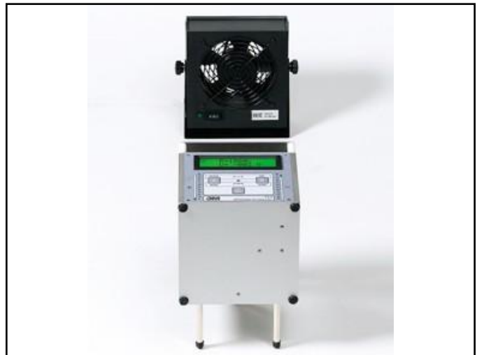
Figure 10. Charge Plate Monitor and Static Decay Time Measurements Using 963E Ionized Air Blower.
